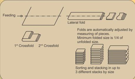
Flexible Lateral folds: Bypass, 1/2, 1/3, 1/4, or fixed size. Flexible Crossfold: Bypass, 1/2, 1/3, 1/4, or fixed size. Three stacking positions for sorted goods.
